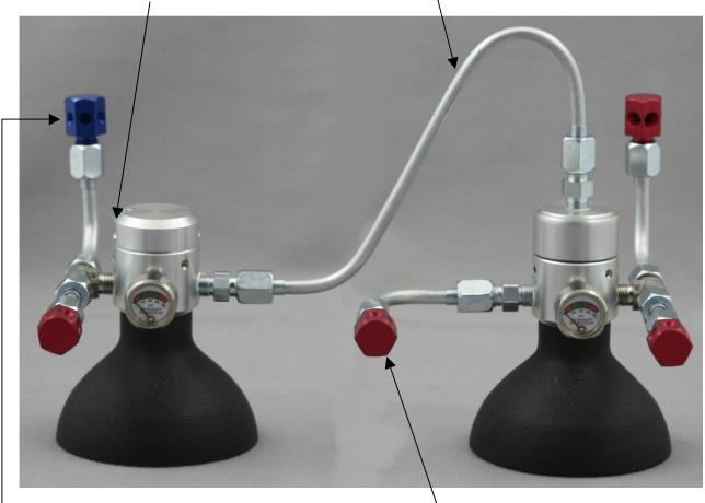
Blue Nozzle – Driver. Run blue nozzle to drivers compartment. Only 1 blue nozzle is needed. Run this nozzle off of pull cable extinguisher Red Nozzles – engine. Run 4 red nozzles to engine compartment
